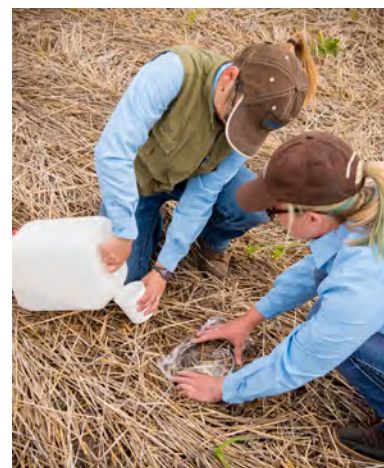
An infiltration test involves driving a 6" ring into the soil, pouring in a known volume of water and recording how long it takes to soak in the ground.
