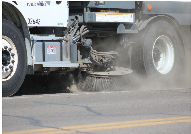
Figure D-9-1. There are different types of street sweeping vehicles, but the most common technology are mechanical broom sweepers, like the one pictured here. More advanced and effective, but expensive, options include vacuum-assisted and regenerative air sweepers (not pictured). Photo: Mississippi Watershed Management Organization
