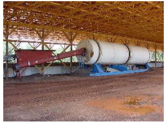
Figure A-14-2. In-Vessel composting is performed in an insulated silo, channel, or bin using a high-rate, controlled aeration system designed to provide optimal conditions. Rotating Drum Composters are a subset of in-vessel composters that aerate compost by turning the compost inside a rotating drum. Photo: Jason Governo, U. of Georgia
