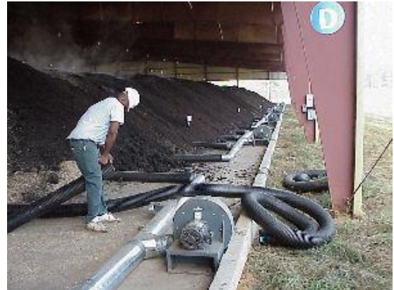
Figure A-14-3. Forced aeration systems, or aerated static piles, use blowers to provide oxygen into the compost pile instead of turning or moving the pile. Photo: Jason Governo, U. of Georgia
